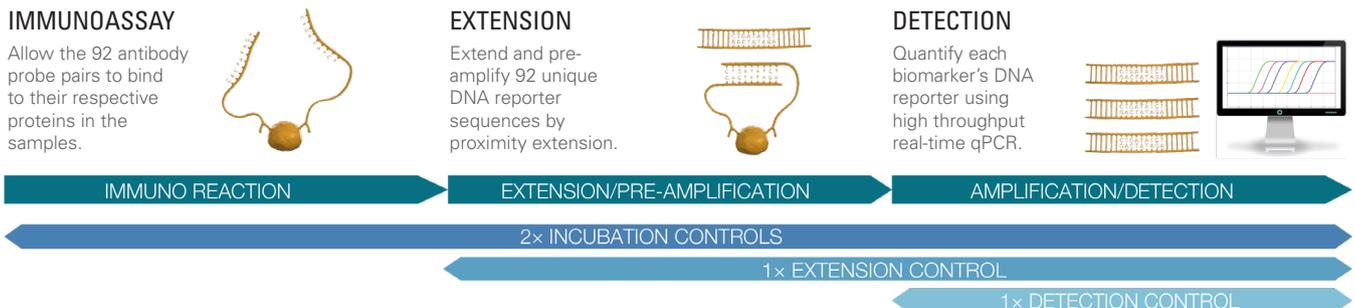
**Fig 1.** Olink assay procedure (above) and controls (below). The internal controls enable monitoring of the three core steps in the Olink assay and used for quality control and data normalization. Detection is performed by using the Fluidigm® Biomark™ or the Fluidigm® Biomark™ HD system.
